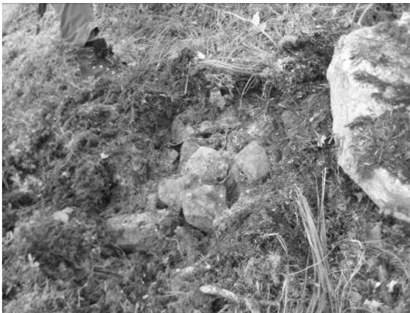
Figure 5.8. Not the moss cover, but the underground hidden under the moss cover is relevant when characterizing the slope surface for a rockfall trajectory study
