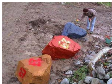
Photo 11 -12 Rocks' preparation and the crane: bio-degradable coloured powder have been used to identified each rock on the numerical films and the rebounds let by he rocks on the ground.
