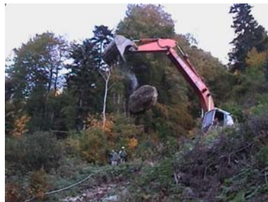
Photo 11 -12 Rocks' preparation and the crane: bio-degradable coloured powder have been used to identified each rock on the numerical films and the rebounds let by he rocks on the ground.
