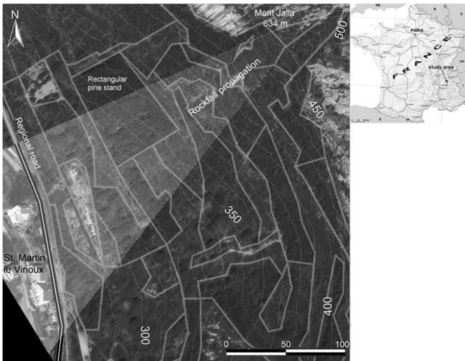
Fig. 3 Map of the study area with the main endangering rockfall zone. The grey polygons represent the polygons mapped in the field. The white numbers indicate the altitude
