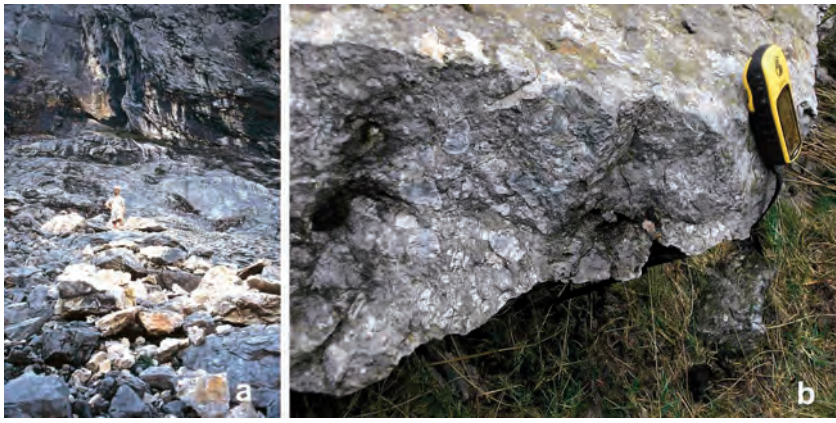
Fig 3 a) Freshly detached surfaces carbonate rocks (Wetterstein limestone) can easily be distinguished optically (Reintal, Bavarian Alps). b) The freshly detached surface of a siliceous volcanic agglomerate with cm-large white inclusions is more difficult to see. The top side on the photo was exposed to weathering prior to the rockfall (Cwm Idwal, Snowdonia, North Wales).
