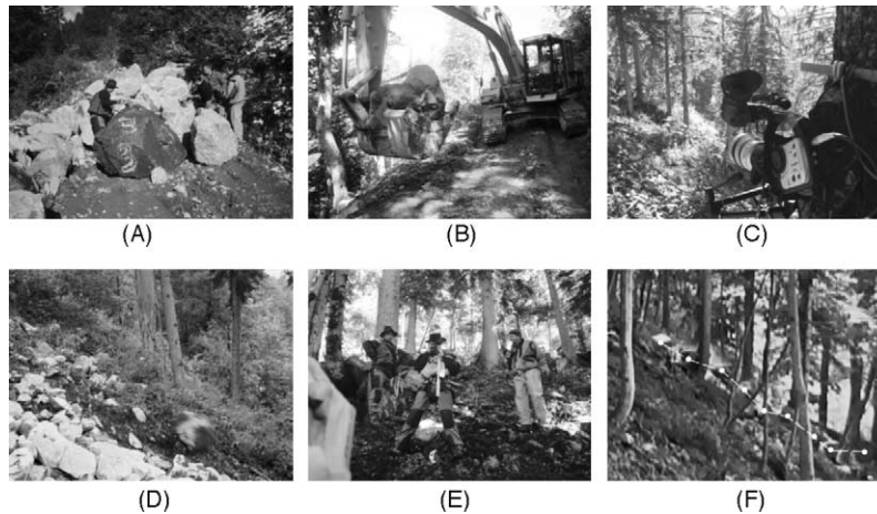
Fig. 2. (A) rocks are painted to leave marks after tree impacts or rebounds on the slope surface; (B) a caterpillar throws the rocks down the slope; (C) video cameras are installed along the slope to record the rockfall trajectories; (D) a rock accelerating in the first meters; (E) after each individual rockfall experiment, we capture its trajectory to obtain a three dimensional trajectory; (F) a sequence of movie images (each 1/4 s) taken at Site 2.
