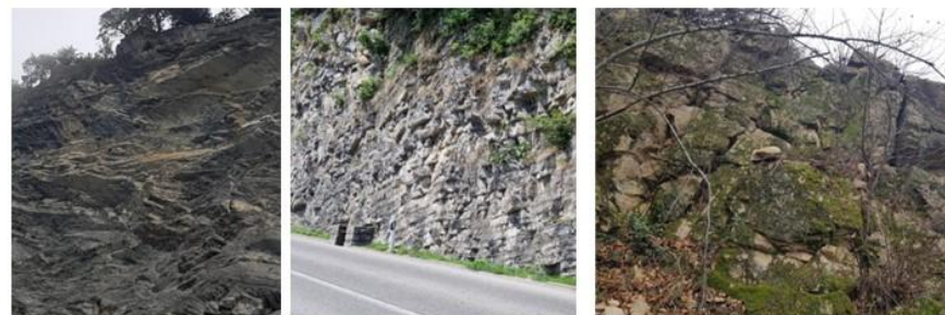
Abb. 8 : Classification of the rock structure for the determination of parameter B. The classes are based on Hoek et al. (2007).
