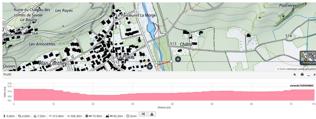
Figure 15: Map showing the stream section selected for the analysis ( https://www.geo.admin.ch ). The red line shows the position of the chosen stream section on the map. The lower panel shows the extrapolated altitude from the digital terrain model along the section.
